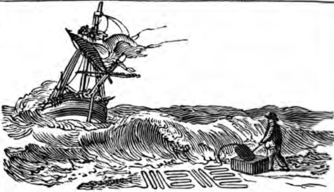
REPRESENTATION OF THE MORTAR, SHOT, AND LINE, PREPARED FOR EFFECTING A COMMUNICATION.
